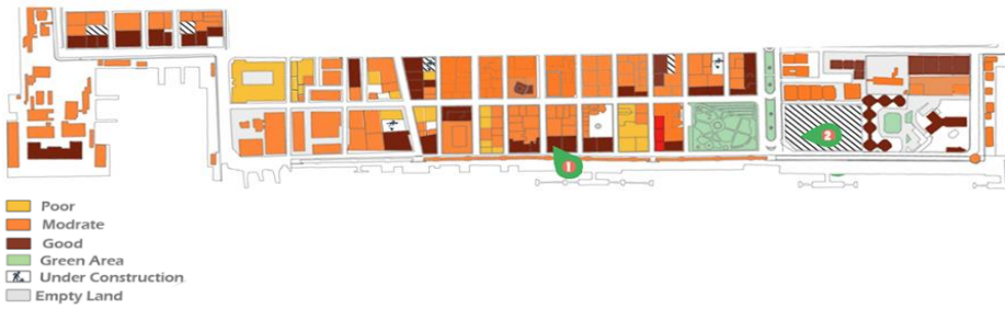
Figure 10: Building Condition study of Palestine Street. Source: developed by the researchers from the site surveying
